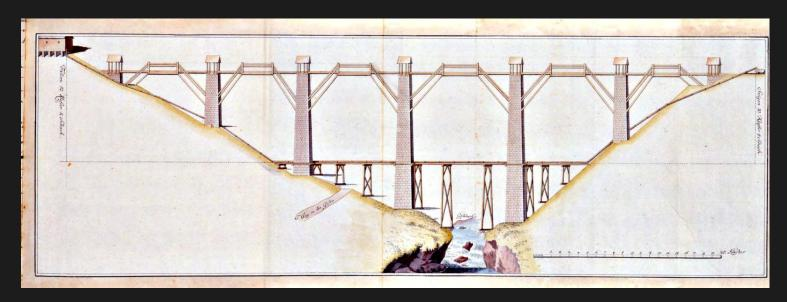
In 1756 it was necessary to build a third brine pipeline next to the two existing ones. During its construction a bridge on up to 30 metres high stone piers was built over the Gosau river, so that the pipeline could slope down evenly. Thus the enormous pressure in the pipes could be reduced a lot, which was a big problem for the technical possibilities at that time.
