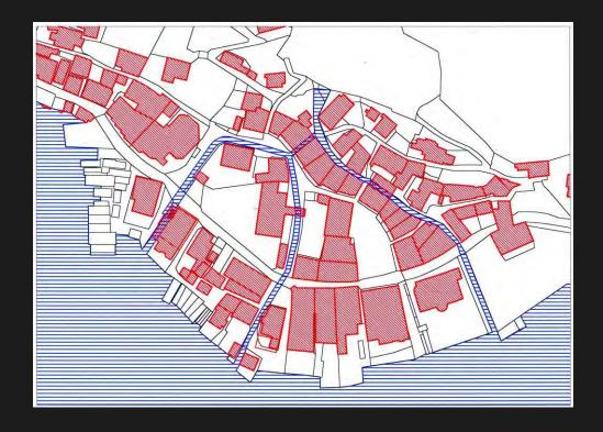
As a result the shapes of the parcels of land are trapeziform and positioned in a way that they do not lay open to the floods and muds of the Mill-brooke that was not regulated before 1888.
