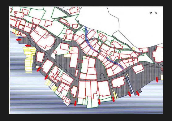
The structure of the paths and docks follows the slope lines and the contour level lines of the alluvial cone. The former main street follows the cone so that the crossing streets are orthogonal to the main street.
