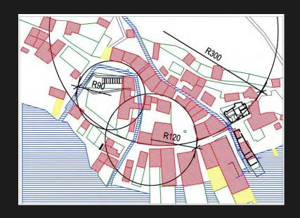
The length of the radius of the circularl main street is exactly 300 "Werkschuh". A "Werkschuh" is a medival local non-metric linear measure.
